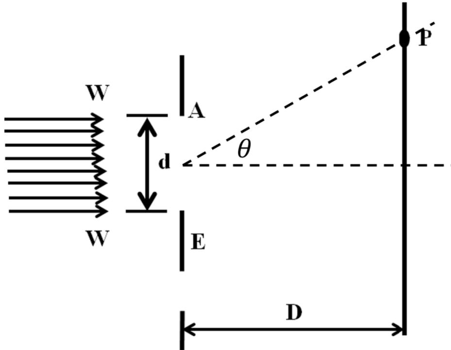
Figure 1: Geometry of the single slit diffraction setup. By
