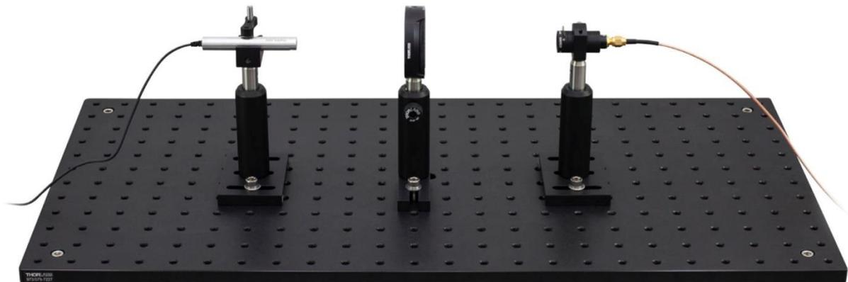
Now rotate the polarizer at an increment size of your choice and measure the photodetector output. The polarization properties of the CPS532-C2 laser modules vary from model to model. Record your measurement and note your findings (in general, the polarization is not linear, but elliptical).
