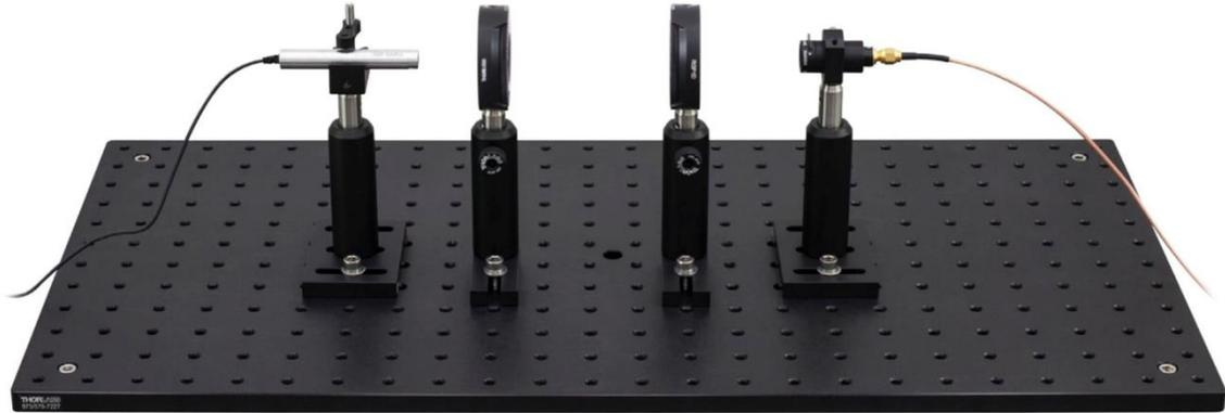
Measure the state of polarization of the laser: Position a polarizer in front of the laser. The photodetector is again positioned behind the polarizer, as shown in the figure below.
