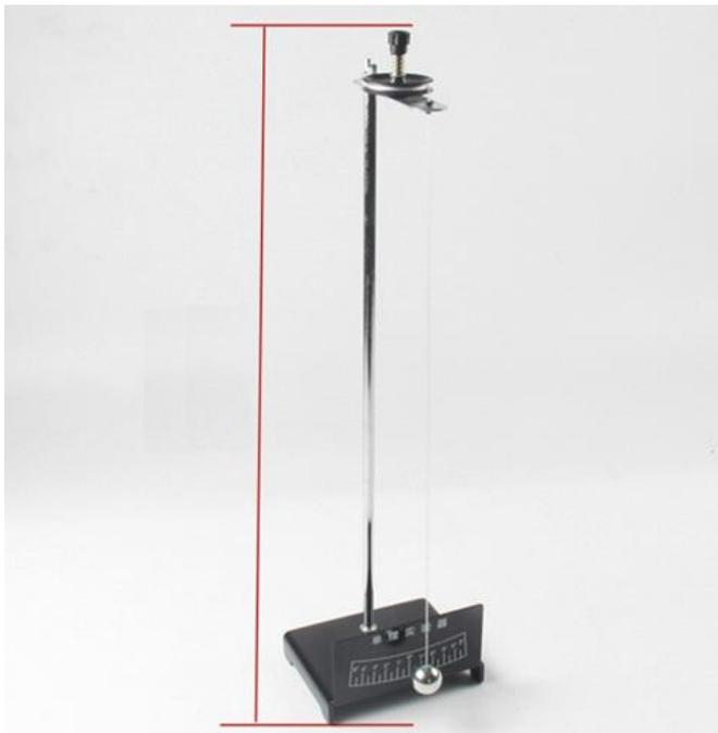
1. Assemble the pendulum by attaching the top end of the string to the pendulum clamp and attaching the pendulum bob to the lower end.
